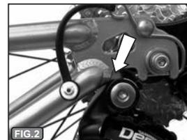
Trailer in extreme counter-clockwise rotation showing contact between derailleur pivot housing and trailer fork. AVOID this condition. If you believe this has occurred, inspect your derailleur, QR, and pins for damage.
