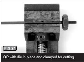
FIG. 24 QR with die in place and clamped for cutting.
