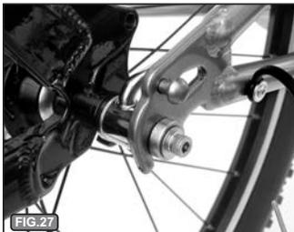
FIG. 27 Fork hooks correctly aligned and installed on bobbins.
