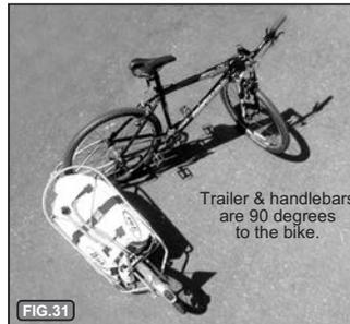
FIG. 31 Parking position. Note: correct direction to turn the handlebars is towards the trailer.
